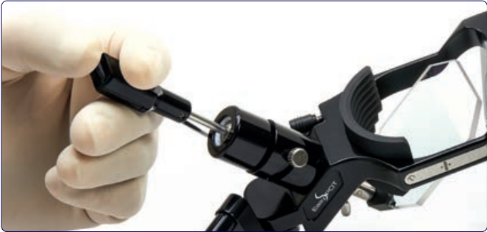
Figure 5. Thanks to the remote control located on the joystick, all the main functions are under the surgeon's direct control without ever taking his eyes off the microscope.
